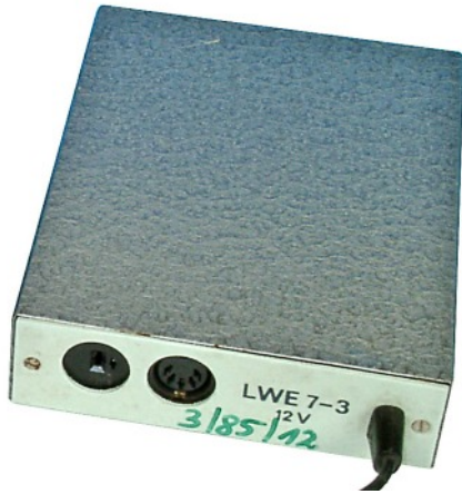
LWE 7-3* 12V receiver (33800*, E7-s) normally used at an Operational Support Point.
